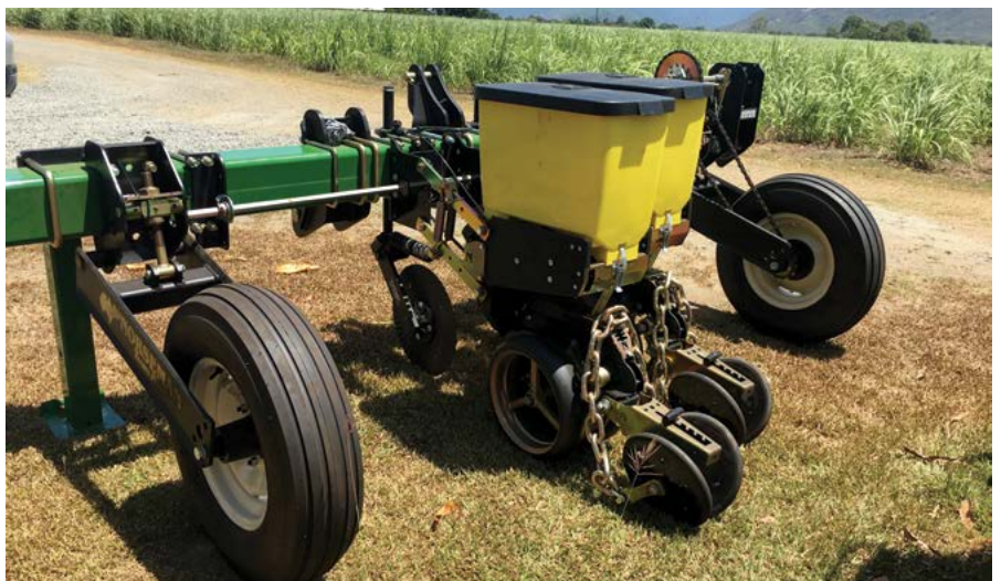
Direct drill bean planter owned by CANEGROWERS Cairns Region.
